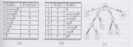
**FIGURE 3.13**: (a) The set of suffixes of S = acacag\$, (b) the corresponding suffix array, and (c) the corresponding suffix tree. Note that the lexicographical order of the leaves in the suffix tree equals the order of the suffixes in the suffix array.
