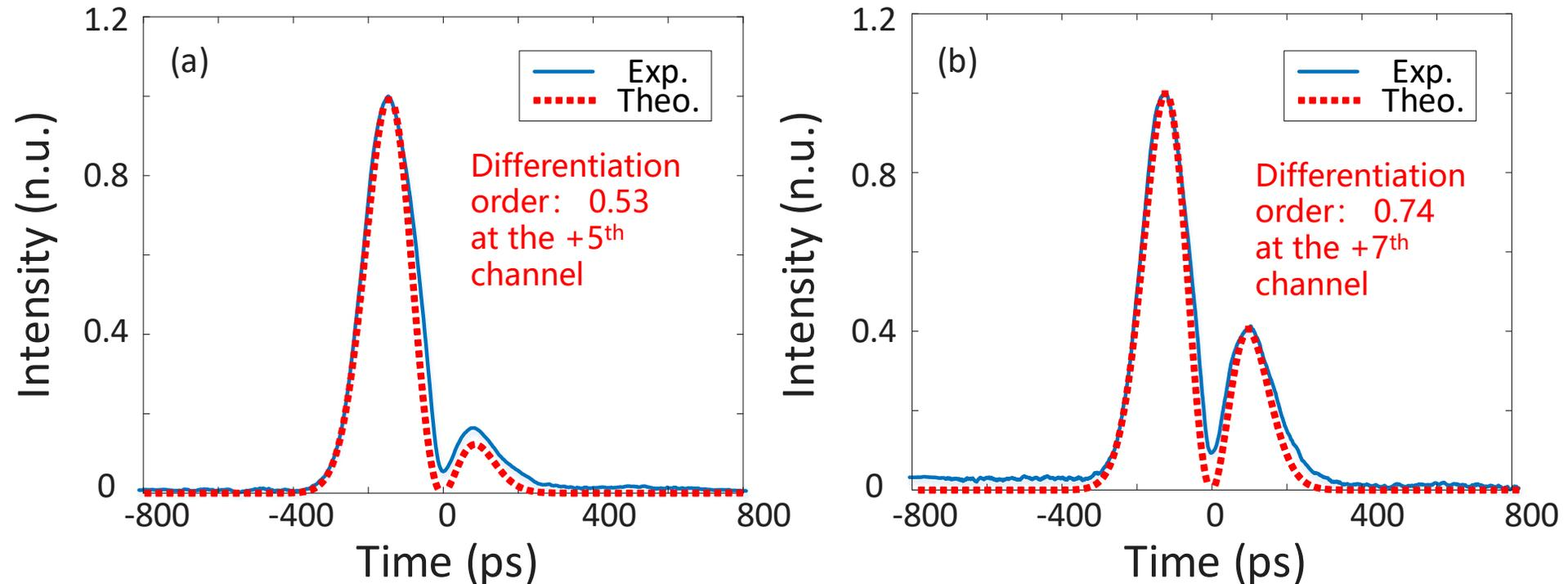
A multichannel temporal differentiator with a channel spacing of 2.4 nm is experimentally demonstrated. The figure shows the measured temporally differentiated pulses corresponding to a differentiation order of (a) 0.53 at the +5<sup>th</sup> channel, and (b) 0.74 at the +7<sup>th</sup> channel.
