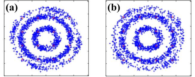
Fig. 19. The measured constellation diagrams of the microwave vector signals at the output of the coherent receiver. (a) The up-converted microwave signal, and (b) The down-converted microwave signal, and.
