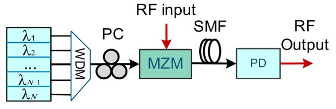
Fig. 10. A delay-line filter using a laser array having multiple wavelengths with an identical wavelength spacing. WDM: wavelength division multiplexer, MZM: Mach-Zehnder modulator, SMF: single-mode fiber, PC: polarization controller, PD: photodetector.
