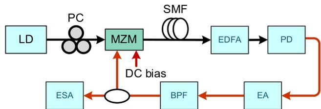
Fig. 4. Schematic of an optoelectronic oscillator (OEO). LD: laser diode, MZM: Mach-Zehnder modulator, SMF: single mode fiber, EDFA: erbium-doped fiber amplifier, PD: photodetector, EA: electronic amplifier, BPF: bandpass filter, ESA: electrical spectrum analyzer.
