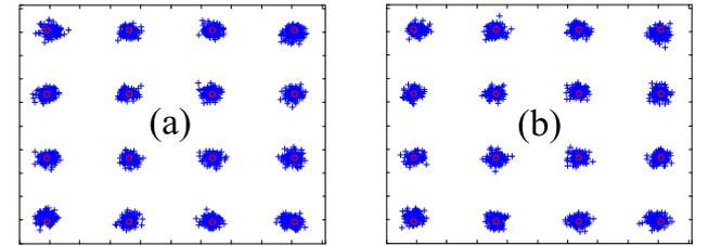
Fig. 20. Constellation diagrams for a recovered 16-QAM microwave vector signal corrupted by an OOK signal through phase modulation, to emulate a strong phase noise applied to the microwave signal. (a) OOK at 1000 Mbps, (c) OOK at 2000 Mbps.
