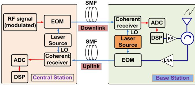
Fig. 16. A duplex RoF link with coherent detection. EOM: electrooptic modulator, SMF: single-mode fiber, ADC: analog-to-digital converter, DSP: digital signal processor, PA: power amplifier, LNA: low noise amplifier, LO: local oscillator.
