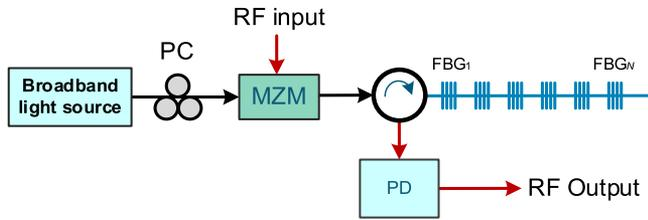
Fig. 9. A delay-line filter using a broadband light source and a fiber Bragg grating array. PC: polarization controller, MZM: Mach-Zehnder modulator, PD: photodetector, FBG: fiber Bragg grating.
