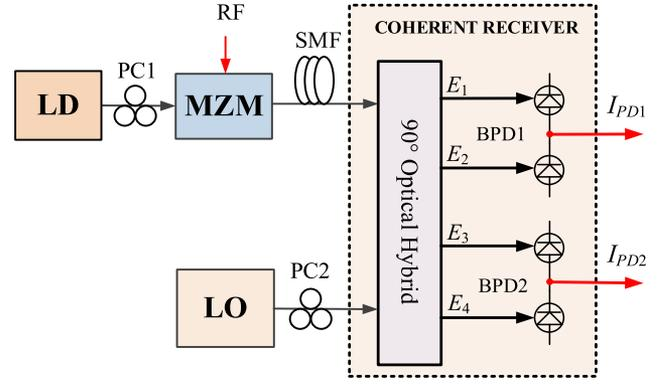
Fig. 17. A coherent RoF link with signal detection at an optical coherent receiver. LD: laser diode, BPD: balanced photodetector, MZM: Mach-Zehnder modulator, LO: local oscillator, PC: polarization controller, SMF: single-mode fiber.
