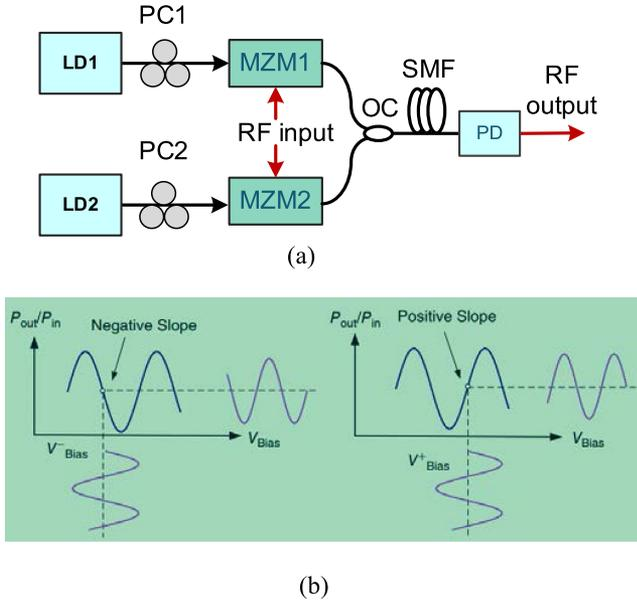
Fig. 11. (a) A two-tap delay-line filter with one negative coefficient. (b) Implementation of negative coefficient by biasing the Mach-Zehnder modulators at the complementary slopes of the transfer functions. LD: laser diode, MZM: Mach-Zehnder modulator, OC: optical coupler, PD: photodetector.
