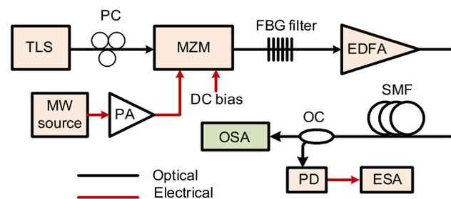
Fig. 3. Microwave signal generation based on external modulation. TLS: tunable laser source, MZM: Mach-Zehnder modulator, OC: optical coupler, SMF: single mode fiber, PA: power amplifier, FBG: fiber Bragg grating, EDFA: erbium-doped fiber amplifier, PD: photodetector, ESA: electrical spectrum analyzer, OSA: optical spectrum analyzer.
