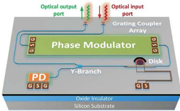
Fig. 13. A silicon photonic integrated microwave photonic filter. [37].
