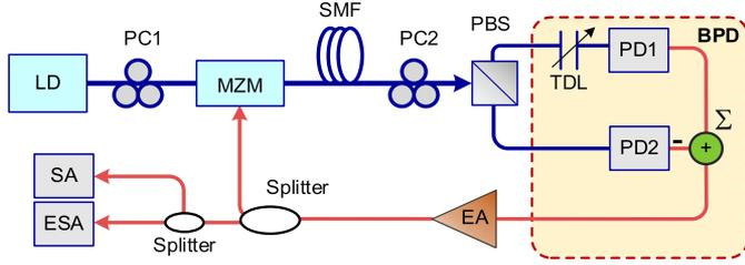
Fig. 6. A parity-time symmetric optoelectronic oscillator. LD: laser diode, PC: polarization controller, MZM: Mach-Zehnder modulator, SMF: single mode fiber, PBS: polarization beam splitter, PD: photodetector, EA: electronic amplifier, ESA: electrical spectrum analyzer, SA: signal analyzer.
