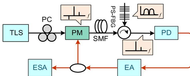
Fig. 5. A frequency-tunable optoelectronic oscillator (OEO) incorporating a frequency-tunable microwave photonic filter. TLS: tunable laser source, PM: phase modulator, PS-FBG: phase-shifted fiber Bragg grating, PD: photodetector, EA: electronic amplifier, ESA: electrical spectrum analyzer.
