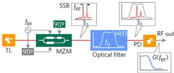
Fig. 14. A monolithically integrated microwave lowpass filter on InP [40].
