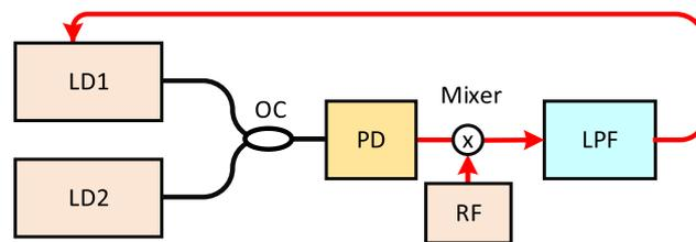
Fig. 2. An optical phase lock loop for low-phase noise microwave signal generation. LD: laser diode, OC: optical coupler, PD: photodetector, LPF: lowpass filter, RF: radio frequency.
