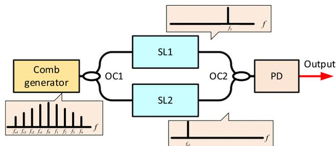
Fig. 1. An optical injection locking system for microwave signal generation. OC: optical coupler, SL: slave laser, PD: photodetector.
