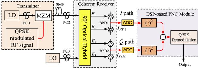
Fig. 18. A coherent RoF link with a DSP-based phase noise cancellation module. ADC: analog-to-digital converter, PC: polarization controller, LD: laser diode, BPD: balanced photodetector, MZM: Mach-Zehnder modulator, QPSK: quadrature phase shift keying.
