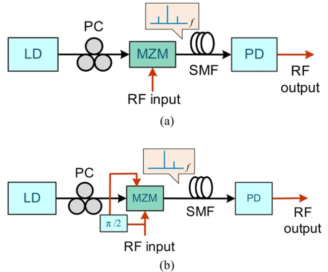
Fig. 15. An IM-DD RoF link. (a) DSB+C modulation, and (b) SSB+C modulation. LD: laser diode, MZM: Mach-Zehnder modulator, SMF: single mode fiber, PD: photodetector.
