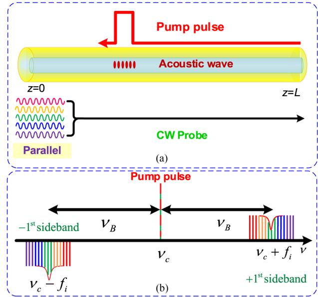
Fig. 21. Principle of an SBS-based distributed microwave photonic sensor. (a) A pump pulse launched into the fiber from the right end, to create SBS effect. A microwave multi-tone signal phase-modulated on an optical carrier is launched into the fiber from the left end. (b) The phase-modulated optical signal is experiencing phase modulation to intensity modulation conversion due to the Brillouin amplification and attenuation to the  $-1^{\text{st}}$  and  $+1^{\text{st}}$  sidebands [51].
