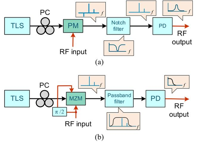
Fig. 12. Microwave photonic filter based on coherent detection. (a) A microwave passband filter implemented based on phase modulation and PM-IM conversion using an optical filter. (b) A microwave lowpass filter implemented based on single sideband plus carrier modulation. TLS: tunable laser source, PM: phase modulator, PD: photodetector, MZM: Mach-Zehnder modulator, PD: photodetector.
