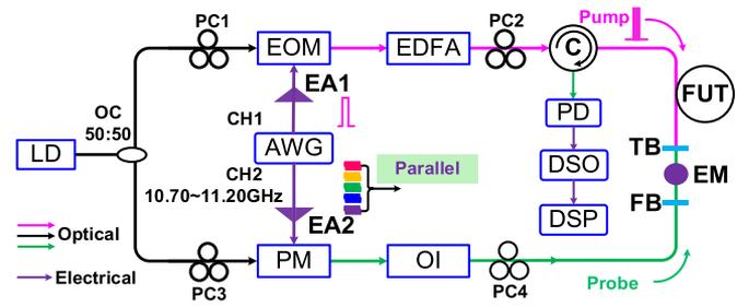
Fig. 22. Schematic diagram of an SBS-based distributed microwave photonic sensor. LD: laser diode, PC: polarization controller, PM: phase modulator, EOM: electro-optic modulator, AWG: arbitrary waveform generator, EDFA: erbium-doped fiber amplifier, OI: optical isolator; FUT: fiber under test, C: optical circulator, PD: photodetector, DSO: digital storage oscilloscope, DSP: digital signal processor, EA: electrical amplifier, EM: electro-motor, FB: fixed base, TB: tunable base [51].
