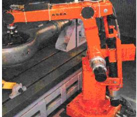
ASEA robot performing mechanical assembly tasks.
