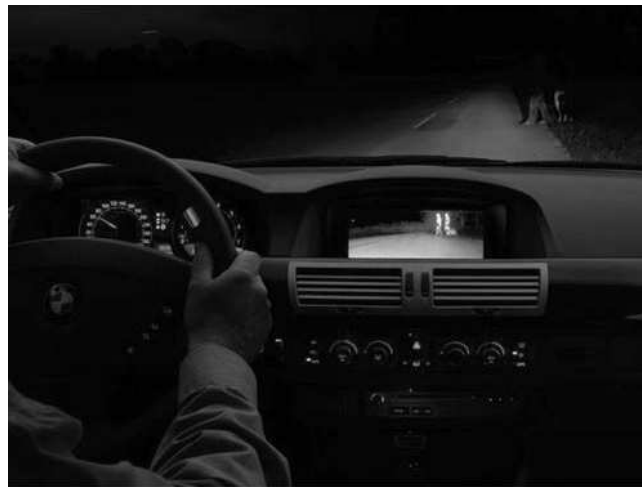
Figure 1.5: The BMW night vision system on a vehicle (courtesy of BMW).
