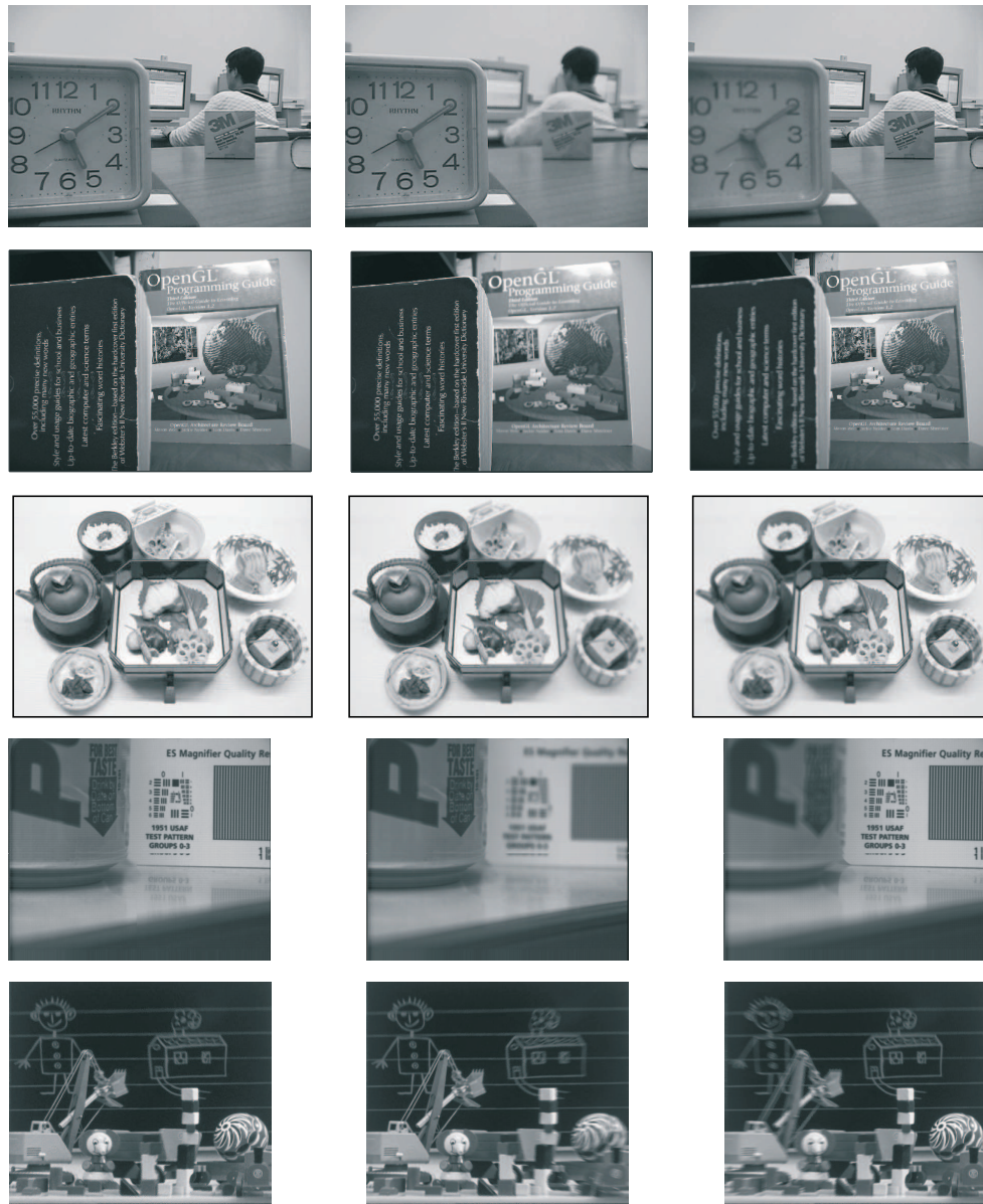
Figure 5.12: The multi-focus images used for the test. From top to bottom: laboratory, books, Japanese food, Pepsi, and object. From left to right: full-focus image, left-focus image, and right-focus image.
