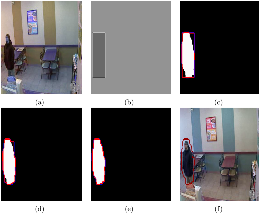
Figure 3.8: Curve evolution procedures. 3.8a shows the original image. 3.8b represents the initial curves and initial level set configuration. 3.8c, 3.8d and 3.8e show the curve evolution with respect to positive F (the pixels with white color). 3.8f final curve.
