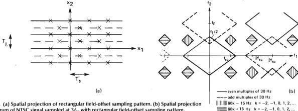
Figure 7. (a) Spatial projection of rectangular field-offset sampling pattern. (b) Spatial projection of spectrum of NTSC signal sampled at  $3f_{sc}$  with rectangular field-offset sampling pattern.
