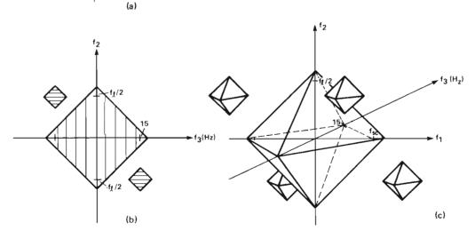
Figure 4. (a) Spatial projection of the basic spectrum of the NTSC color signal. (b) Vertical-temporal projection of the basic spectrum of the NTSC color signal. (c) Perspective view of the basic spectrum of the NTSC color signal.
