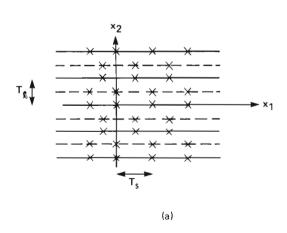
Figure & (a) Spatial projection of checkerboard sampling pattern. (b) Spatial projection of spectrum of NTSC signal sampled at 3fsc with checkerboard samp ling pattern.
