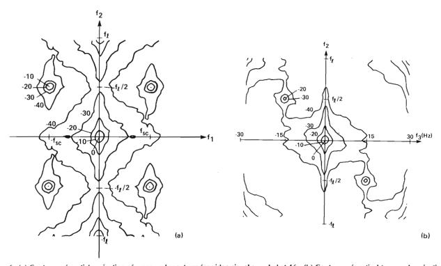
Figure 6. (a) Contours of spatial projection of measured spectrum for video signal sampled at  $4f_{sc}$ . (b) Contours of vertical-temporal projection of measured spectrum for video signal sampled at  $4f_{sc}$ . Relative power in decibels shown on selected contours.
