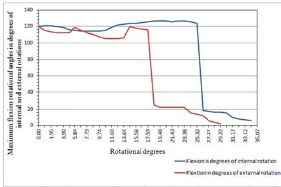
Fig. 8. Maximum flexion rotational angles ( ^{\circ} ) of hip joint in degrees of external and internal rotations.
