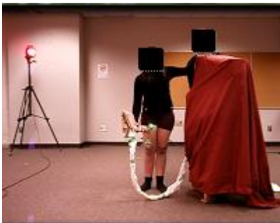
Figure 1 : Setup with participant handling the ultrasound probe. Ultrasound machine was covered with cloth to avoid reflections and VICON camera
