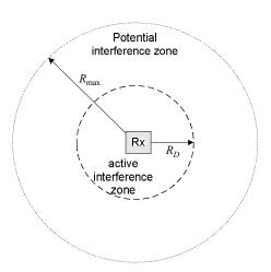
Fig. 2. Interference zones on the network scale. Potential interference zone:  $R \le R_{\text{max}}$ ,  $P_a(R) \ge P_0 = P_a(R_{\text{max}})$  (the signal power exceeds the Rx noise level); active interference zone:  $R \le R_D$ ,  $P_a(R) \ge P_{df} = R_a(R_D)$  (the signal power exceeds the maximum distortion-free power)
