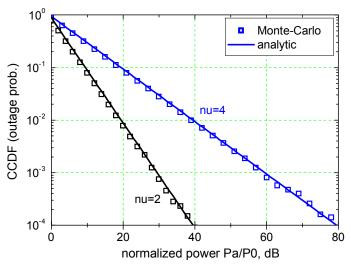
Fig. 3. The CCDF of  $P_a/P_0$  evaluated from Monte-Carlo (MC) simulations (10<sup>5</sup> trials) and from (15) for *m*=2, v=2&4
