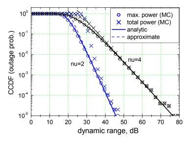
Fig. 6. The CCDF of  $d_a = P_{a1}/P_0$  and  $d_{tot} = P_{tot}/P_0$  with the most powerful signal cancelled (*k*=2), evaluated from MC simulations (10<sup>5</sup> trials) and from the analysis, for *m*=2, v=2&4,  $P_0=10^{-10}$ ,  $P_t=1$ ,  $\rho=10^{-5}$ . Significant improvement over the *k*=1 case is clear
