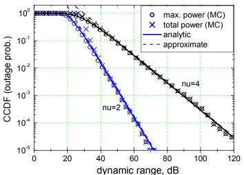
Fig. 5. The CCDF of  $d_a = P_{a1}/P_0$  and  $d_{tot} = P_{tot}/P_0$  (i.e. the outage probability) evaluated from Monte-Carlo (MC) simulations (10<sup>5</sup> trials) for m=2, v=2&4,  $P_0=10^{-10}$ ,  $P_t=1$ ,  $\rho=10^{-5}$ ; analytic CCDF of  $d_a$  (derived from (26)) and its approximation in (34) are also shown
