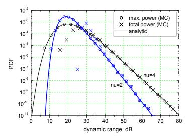
Fig. 4. The PDF of  $d_a = P_{a1}/P_0$  and  $d_{to} = P_{tot}/P_0$  evaluated from Monte-Carlo (MC) simulations (10<sup>5</sup> trials) for m=2, v=2&4,  $P_0=10^{-10}$ ,  $P_t=1$ ,  $\rho=10^{-5}$  and analytic PDF of  $d_a$  (see (26))
