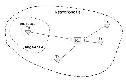
Fig. 1. Illustration of the problem geometry and three associated scales: small-scale (immediate neighborhood of a Tx; this is the scale of multipath fading), large-scale (extends beyond immediate neighborhood but is smaller than the whole network area; this is the scale of shadow fading) and network-scale (includes the whole network; this is the scale of network fading in (11)-(15)).
