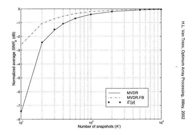
Figure 7.4 MVDR SMI beamformer:  $\bar{\rho}$  and  $E[\rho]$  versus K.
