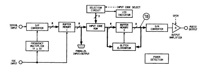
Figure 2. Block Diagram of the PCM Decoder.
