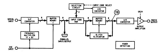
Figure 3. Location of the Test Bus.
