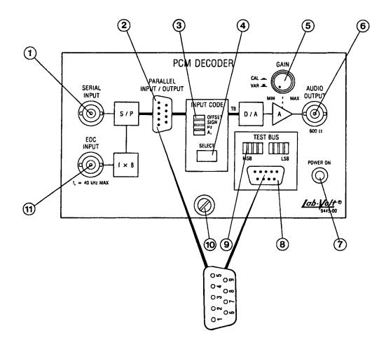
Figure 1. Front Panel of the PCM Decoder.
