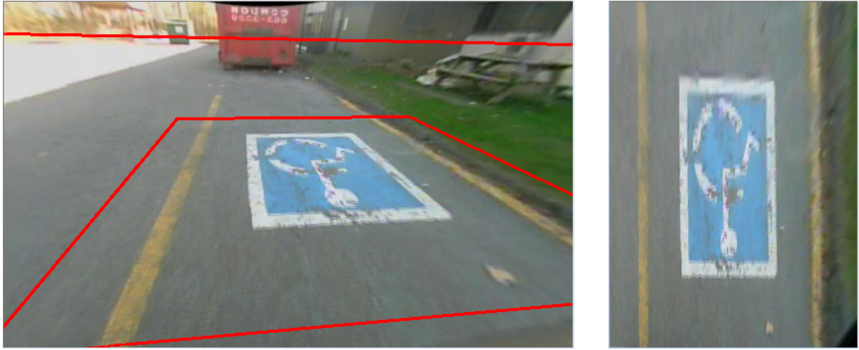
Figure 7.1: Manual camera orientation estimation from a bird's eye view. The bird's eye view (right) taken from the dewarped image (left) is produced by manually selecting the camera orientation w.r.t. the ground.
