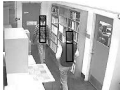
Fig. 2 A sample image showing two detected persons and the regions of interest.
