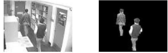
Fig. 1 Example of silhouette formation. (a) A sample image. (b) The silhouette formed using background comparison.
