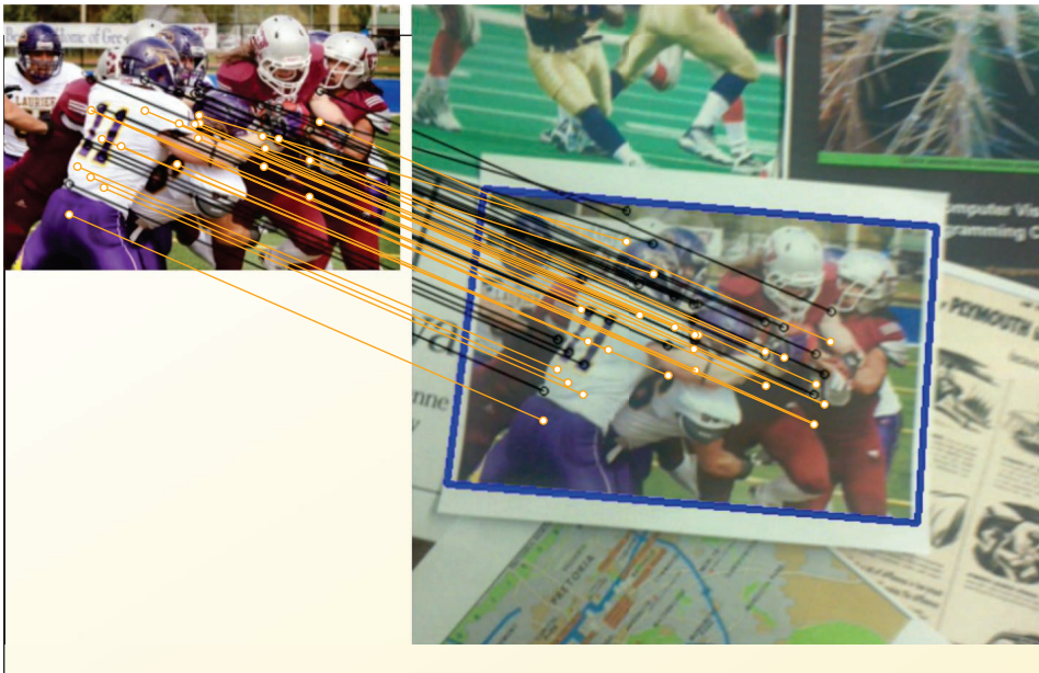
Fig. 4. Matching of local features between a target and an image of it.
