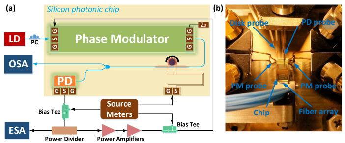
Fig. 1 (a) Schematic of the proposed integrated frequency-tunable OEO on a silicon photonic chip. LD: laser diode LD, PC: polarization controller, OSA: optical spectrum analyzer, ESA: electrical spectrum analyzer; (b) a picture of the text set-up.
