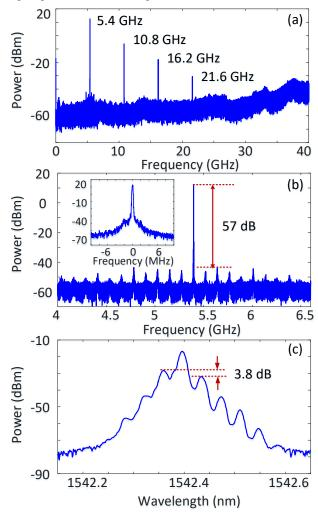
Fig. 3 (a) Electrical spectrum of the generated 5.4 GHz signal (the frequency span is 40 GHz and the resolution bandwidth (RBW) is 200 KHz); (b) electrical spectrum with a frequency span of 4 GHz and a RBW of 200 KHz. Inset shows a zoom-in view of the electrical spectrum with a frequency span of 20 MHz and a RBW of 180 KHz; (c) measured optical spectrum at the optical output grating coupler when the OEO is operating at 5.4 GHz.
