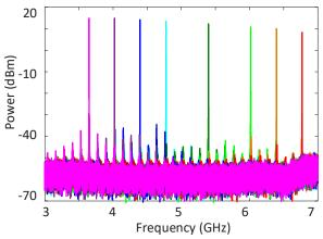
Fig. 4 Measured electrical spectrums of the generated microwave signal at different frequencies. The frequency is coarsely tuned from 3 to 7 GHz and the RBW is 200 KHz.
