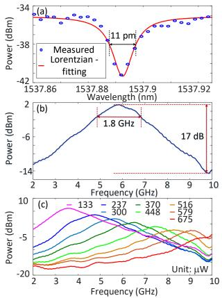
Fig. 2. (a) Measured magnitude response of the MDR; (b) measured frequency response of the MPF with a center frequency of 5.84 GHz; (c) measured frequency responses of the MPF with its center frequency tuned from 3 to 7 GHz.
