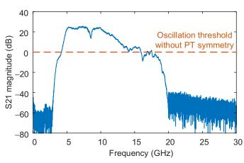
**Fig. 3. S21 magnitude response of the OEO with only one loop closed.** It is measured by a vector network analyzer (VNA) connected between the MZM and the EA with the measurement direction indicated in Fig. 1.
