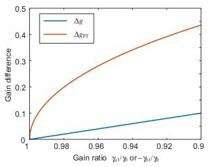
**Fig. 2. Gain difference enhancement with PT symmetry.** The gain difference between the oscillating mode and the secondary mode within a regular single-loop OEO (blue) and a PT-symmetric OEO (red) is illustrated for comparison.
