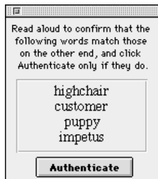
Figure 4D: PGPfone "voice signature" mechanism.
